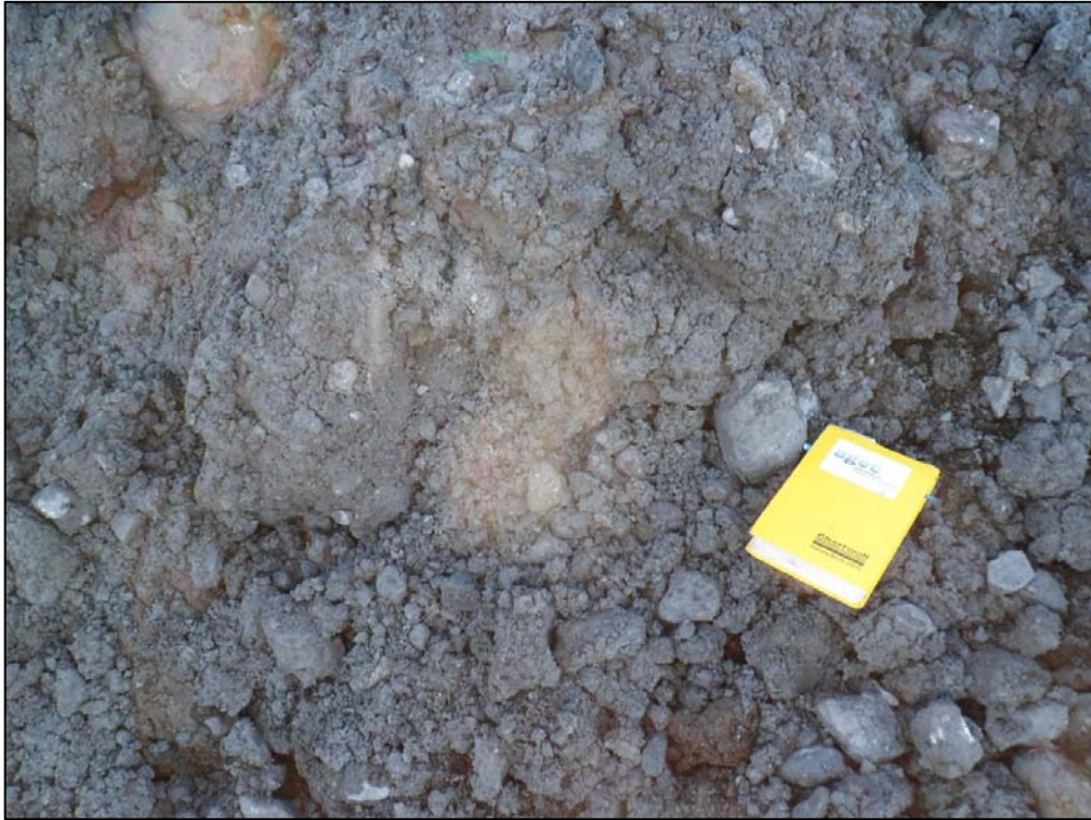
Photo 17 Excavated arisings from trial pit TP14
